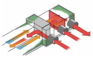
The Clima<sup>+</sup> 200 can be used as a complete heating system by extending it with a heating unit. This heater in combination with recirculation of air enables you to control the temperature inside the poultry house regardless of the weather conditions. The heater can be integrated in the Clima<sup>+</sup> 200 and thereby makes heaters inside the house redundant. The complete heating system enables you to create perfect and constant climate conditions for optimal bird performance.
