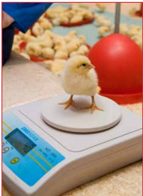
Figure 57: Electronic platform scales for individual bird weights up to 7 days of age.
