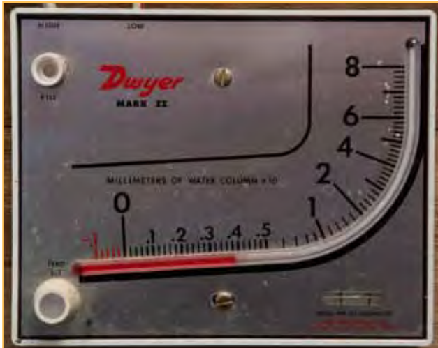
Figure 103: A manometer used to monitor air pressure within the house (the reading given is equivalent to 37.5 Pa).
