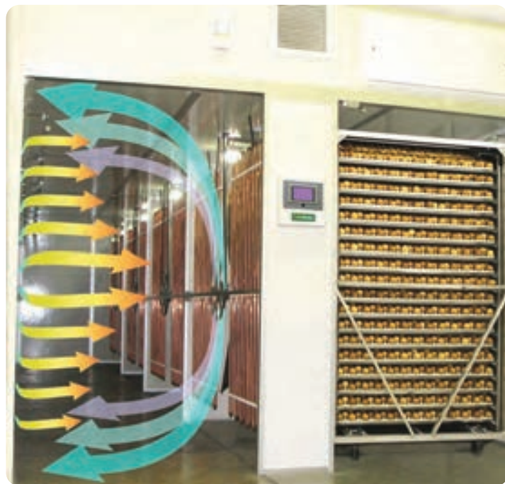
Uniform airflow creates the perfect micro climate around each egg
