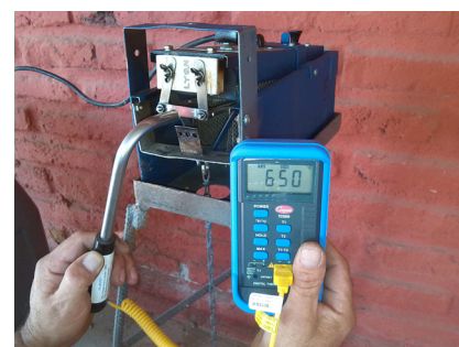
Pyrometer indicating proper blade temperature of 650°C.
