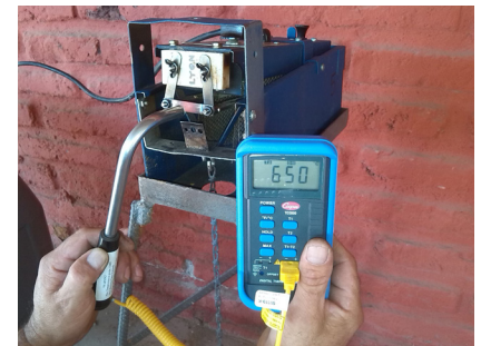
Pyrometer indicating proper blade temperature of 650°C.
