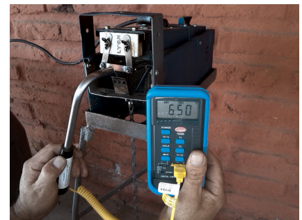
Pyrometer indicating proper blade temperature of 650°C.
