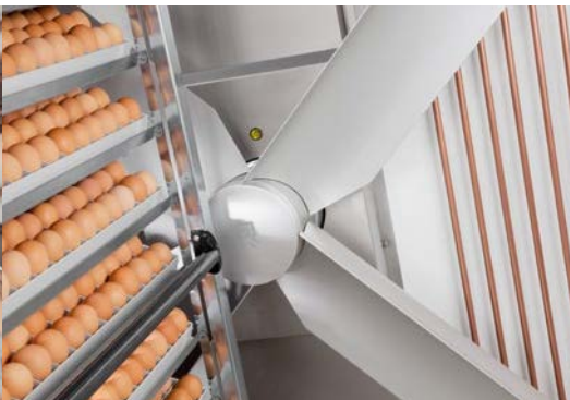
Vortices flow parallel with turning direction of trays
