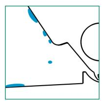
The air inlet uses the Venturi effect to draw in the air inside the house along with the incoming air. The round opening keeps the air in the house moving to prevent condensate from forming on the valve. The blunt corner on the inside of the valve and the slanted edge of the lower corner sections cause the condensate to run off the moving parts.
