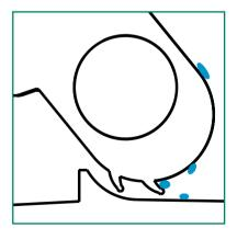
Two rubber strips seal the lower side of the valve to prevent the condensate from dripping into the moving parts and air from leaking away under the valve.
