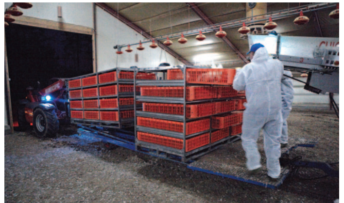
Rotating platform on trailer.
