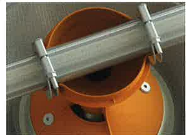
Openings (at the top and the bottom) facilitate a thorough cleaning
